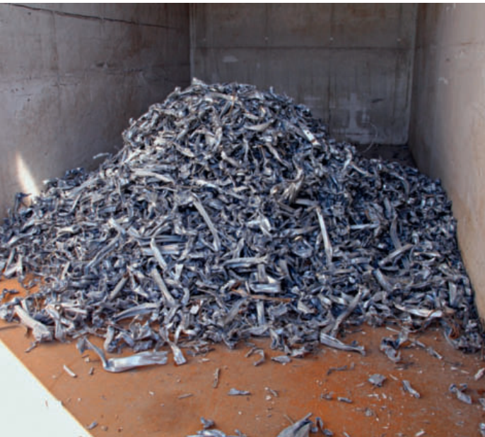
▲ Ferrous-metals scrap separated out from window recycling
