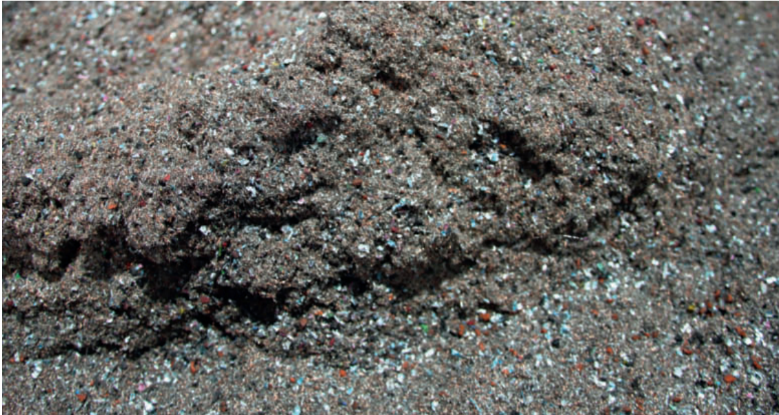
▼ 3 Fines fraction recovered from metal composites
