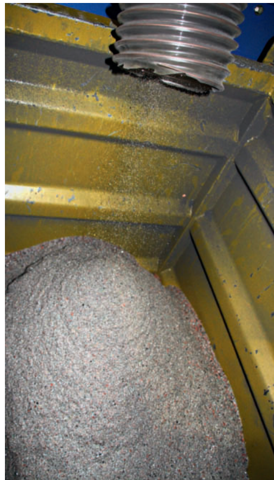
◀ 4 Metal fines fraction from density-based sorting
