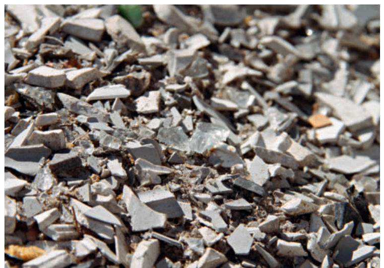
▼ The fine fraction screened off contains the minerals and glass
