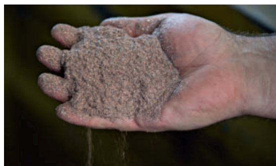
▲ 9 Copper/aluminium fines fraction as the sample material for the tests
