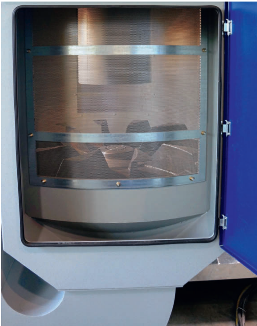
4 View through a tangential screen into the centrifuge compartment of the DRD 26 system. At the bottom you see the double rotor system with 12 rotor blades, above them there is the casing of the heating damper
