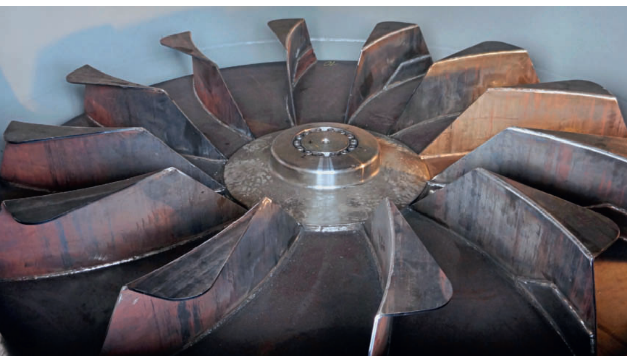
◀ 2 The "dual" rotor is the central system component of the DRD system. The suction end for the feed is on the bottom side, which cannot be seen here
