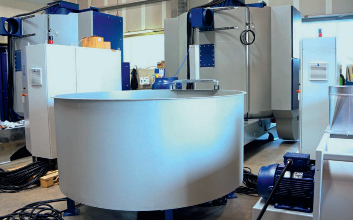
◀ 1 Two DRD 26 plants being set up. In the foreground you see a buffer bin for the material feed, in the background there are the centrifuge compartments including electrical and control console
