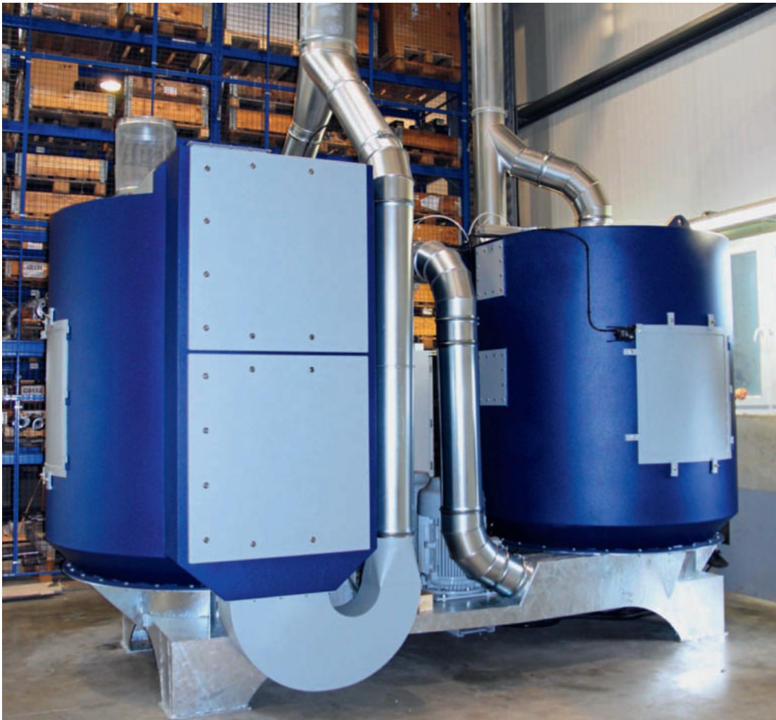
7 Two-stage plant DRD 21 DS. On the left there is the first cleaning stage including heating damper, on the right there is the second one operating without air heating
