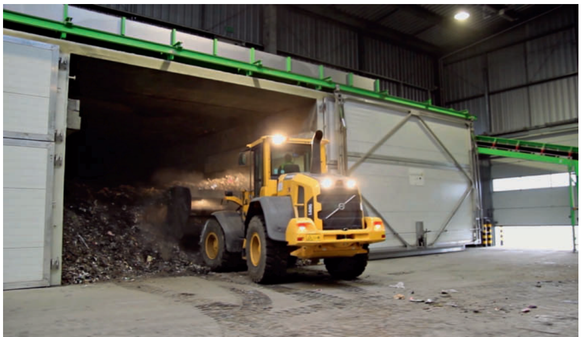
Emptying of the rotting tunnels ▶
